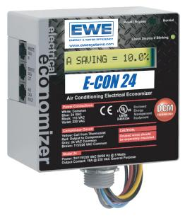
*E-con* is a microprocessor-based, electricity-saving control for commercial air conditioning systems. *E-con* 24 reduces compressor run time, excessive cycling and electrical usage, when installed on any new or existing air conditioning compressor. E-con 24 uses intelligent Dynamic Cycle Management (DCM) technology to save energy by adjusting the compressor run pattern to match the system's "cooling load".
